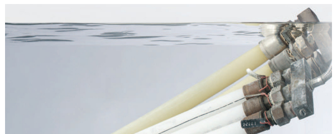
Pipes in a long-term test (under pressure in a water bath)
