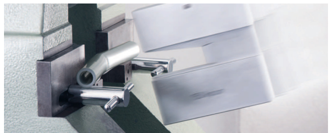
Universal pipe RAUTITAN Flex in the notch impact testing device
